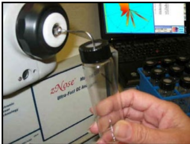
Figure 5- Analyzing the chemical signature of headspace vapors from soap and lotion
