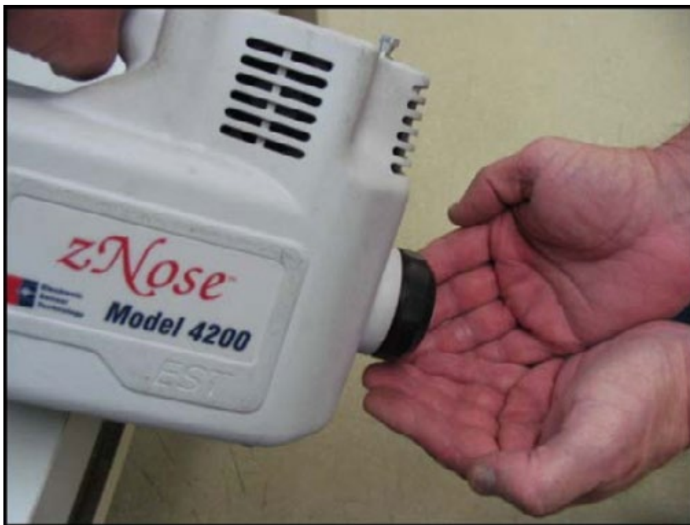
Figure 10- Using zNose® to test chemical vapors associated with use of antiseptic soaps and lotions
