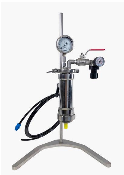
Figure 2: 0.2L Nutsche that was used for the experiments in Figs. 5-8.
