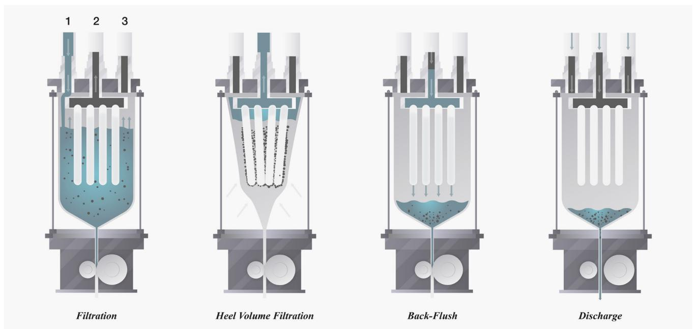
Figure 1: Filtration steps that comprise one complete cycle of the CONTIBAC SU® <sup>[3]</sup>.
