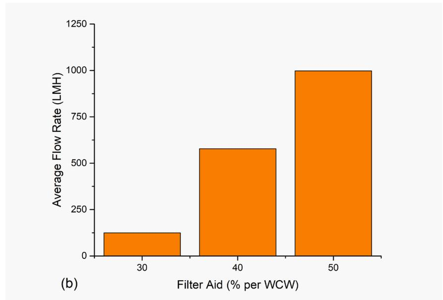
**Figure 6:** Average flow rates over (a) 200 ml and (b) 100 ml suspension volume, which yielded a cake thickness near 10 mm in both cases. The experiments in (a) were performed with cell culture 1 and the fine filter medium. The experiments in (b) were performed with cell culture 3 and the coarse medium. In both experiments the pressure was set to 1.5 bar.
