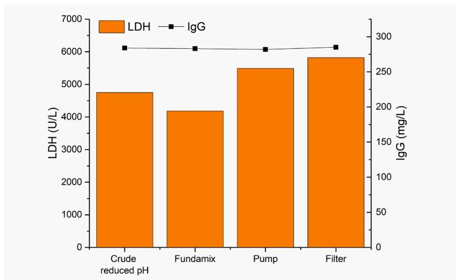
Figure 9: Amount of cell debris (LDH) and product (IgG) measured at different steps of the filtration setup. The tests were performed with cell culture 2, 40% filter aid per WCW, the fine filter medium, and a pH of 4.9. The activity of LDH value after the FUNDAMIX® is lower than the activity of LDH value of the crude harvest due to measurement uncertainties.
