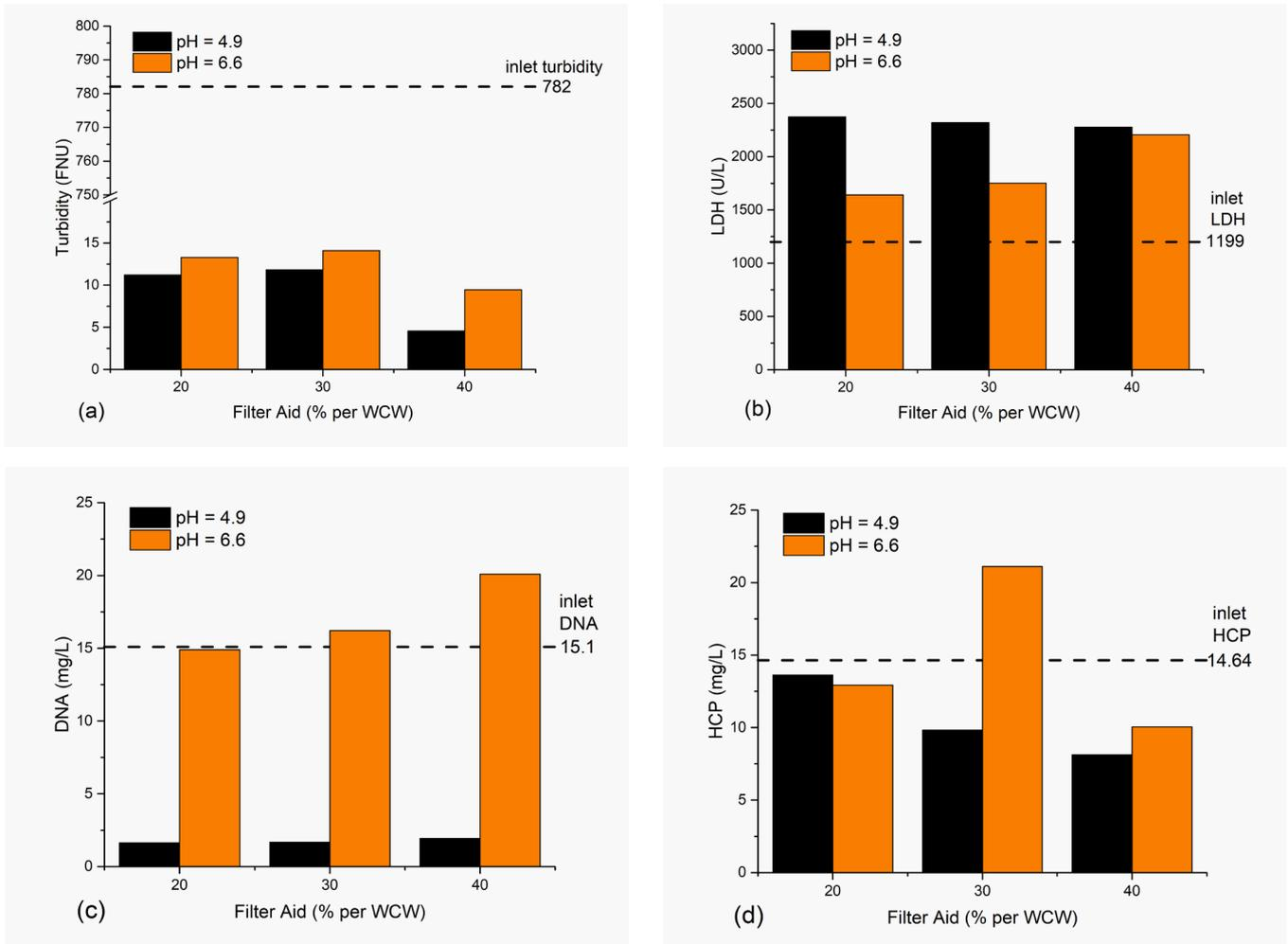
Figure 8: (a) Turbidity, (b) activity of LDH, (c) DNA, and (d) HCP measurements at the crude pH and a reduced pH for 20 – 40% filter aid per WCW. The experiments were performed with cell culture 1 and the fine filter medium. The dashed line shows the corresponding inlet values.
