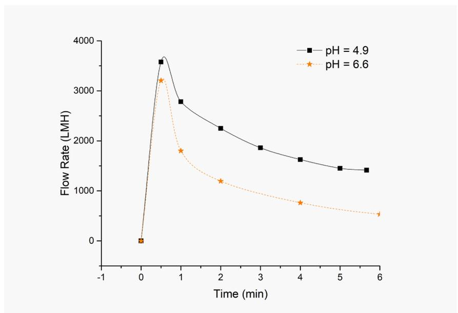
Figure 5: Flow curves at 40% filter aid per WCW. The experiments were performed with cell culture 1 at a pressure of 1.5 bar. The flow rate is given in terms of liters per square meters per hour (LMH).
