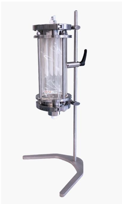
Figure 3: 2L CONTIBAC® SU that was used in Fig. 9 and Table 2.
