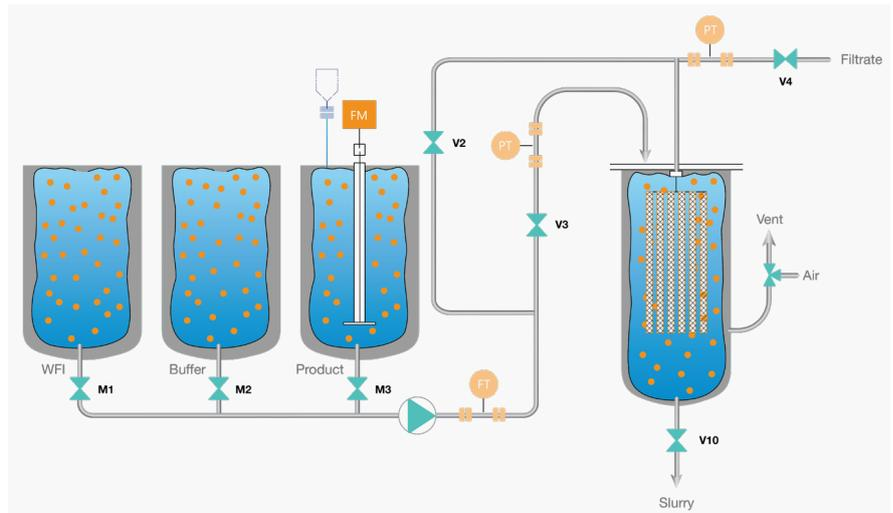
Figure 4: Schematic of the CONTIBAC® SU filtration setup.
