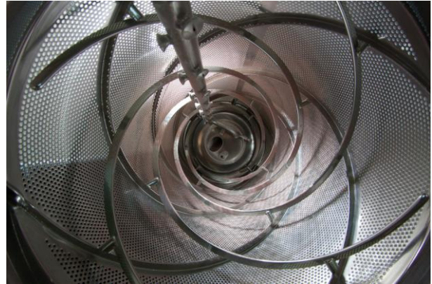
Figure 6 View into the coating pan after eight coating cycles. As can be seen, no major deposits are visible.
