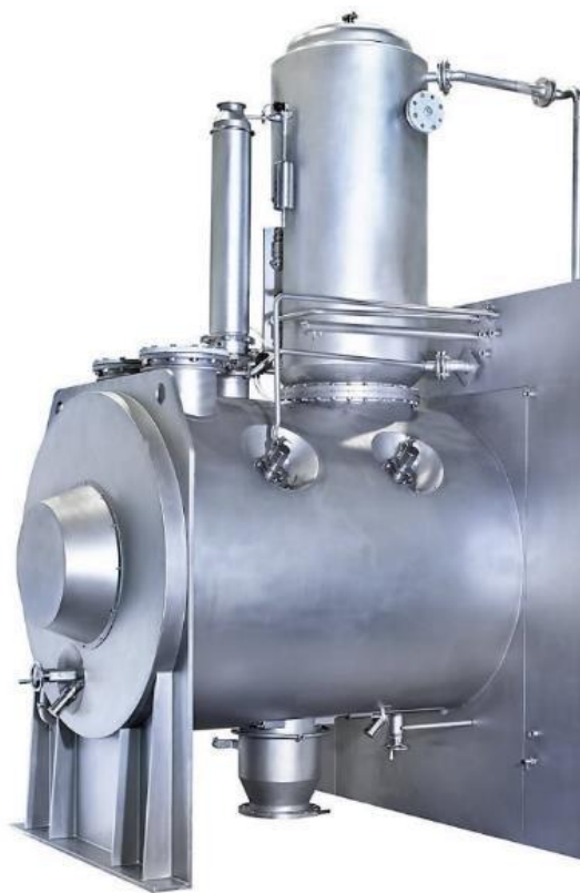
Fig. 5: Horizontal single-pot device for production purposes [4]
