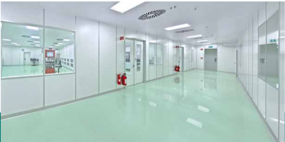
The pharmaceutical packaging and filling area can be flexibly divided into units. It is comprised of three classified and certified clean rooms according to GMP class D (ISO 8) of between 70 and 90 sqm.
